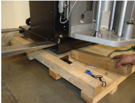
Insert 2X4 underneath frame to raise up
