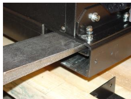
Raise forks to lift frame from base
