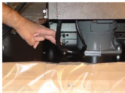
Push tower upward into up right position.
