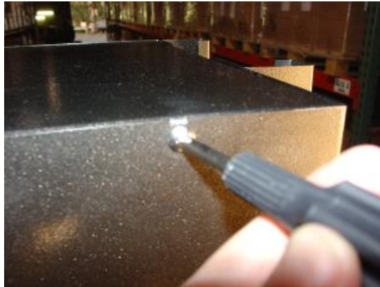
Remove top cover on tower mast
