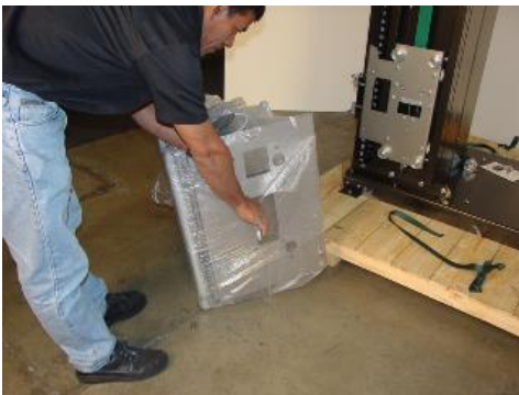
Remove plastic from pre-stretch Assembly
