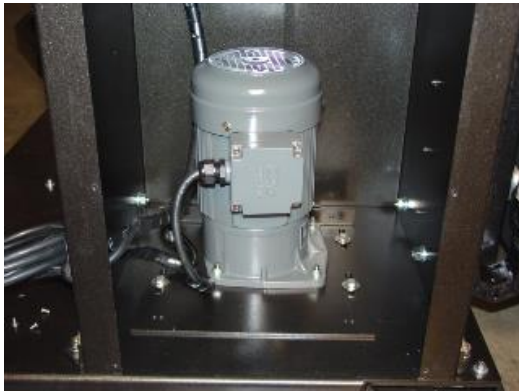
Motor mounts are slotted and allow greater adjustment of chain tension.
