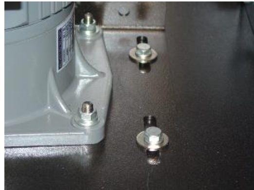
Motor mounts are slotted and allow greater adjustment of chain tension.
