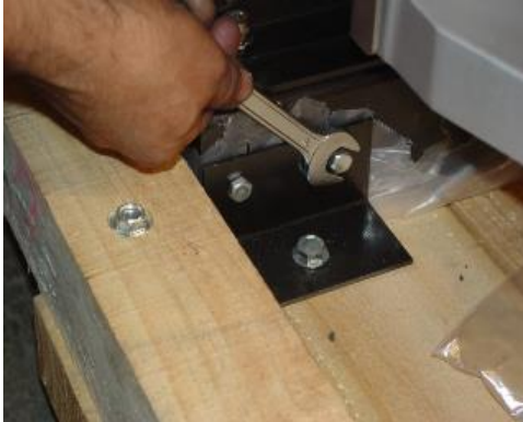
1. Remove the 2 bolts from Holding plate near tower base On both sides of machine
