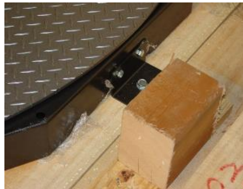
2. Remove 2 bolts from holding plate at opposite end of machine near turntable
