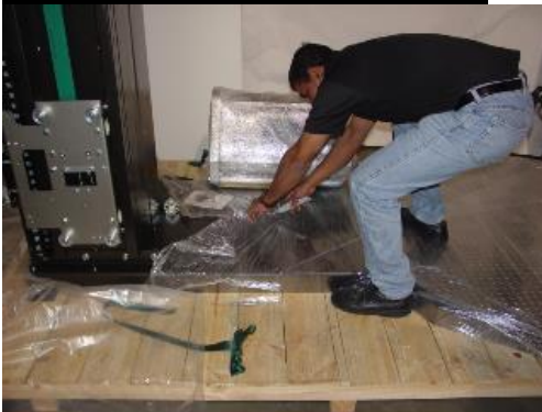
Remove plastic covering from Base and turntable.
