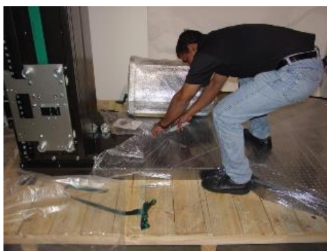
Push tower upward into up right position.
